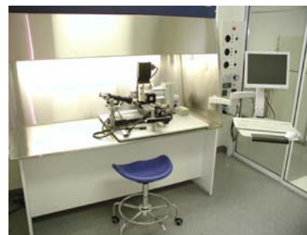
Fig. 2: Desktop JetLab ® system attached to a tissue culture hood for sterile manufacturing.
