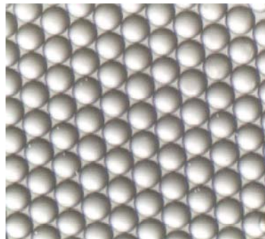
Fig. 3: PLGA paclitaxel-loaded jetted microspheres (100 \mu m after jetting, 50 \mu m after curing).
