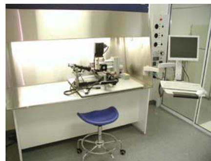
Fig. 2: Desktop JetLab<sup>®</sup> system attached to a tissue culture hood for sterile manufacturing.
