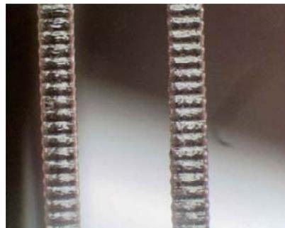
Fig. 8: Nerve conduits manufactured by valve-jet technology.
