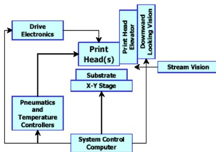
Fig. 1: JetLab<sup>®</sup> system block diagram.
