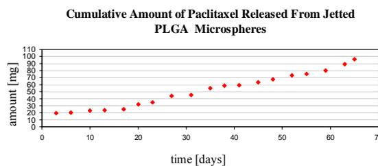
Fig. 5: Release kinetic profile of paclitaxel from jetted microspheres.
