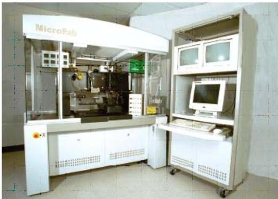
**Figure 4.** JetLab® printing station for direct writing from data files of patterns and consisting of 4 printheads, XYZ &  $\theta$  stages, UV-curing head, N<sub>2</sub> co-flow, pneumatic & temperature controls, and software.
