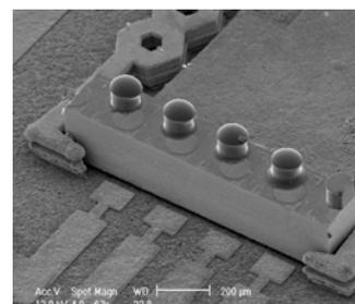
**Figure 25.** A lensed VCSEL die is positioned by a MEMS clamper.
