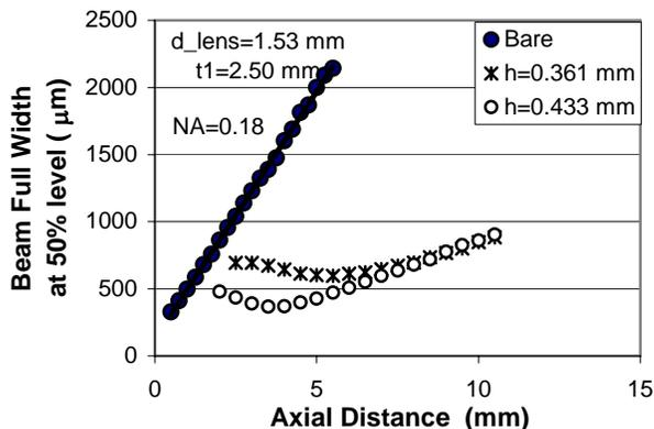
**Figure 12.** Beam width vs. axial distance of lensed sensor-grade fiber.
