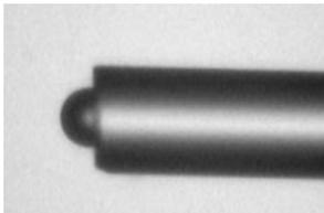
**Figure 8.** A 70 μm diameter microlens printed onto the tip of a 125 μm diameter optical fiber to increase NA.
