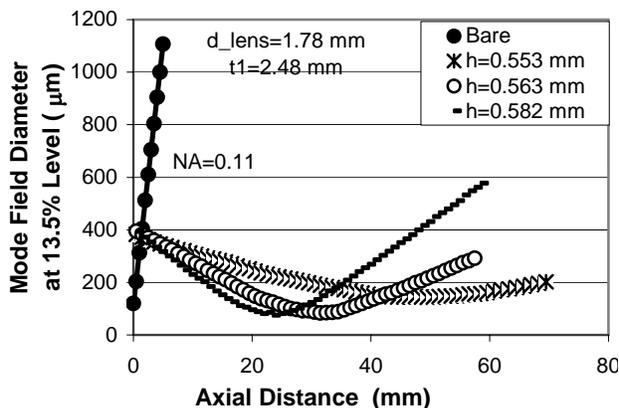
**Figure 11.** Beam width vs. axial distance of lensed single mode fiber.
