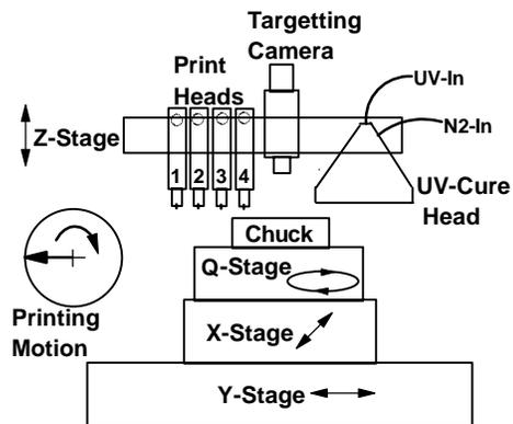
**Figure 5.** Schematics of layout of key elements of printing station and of simultaneous use of rotary and linear motions.
