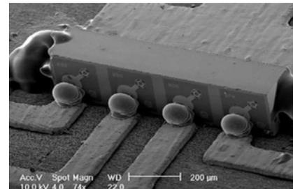
**Figure 20.** Direct VCSEL die bonding using SolderJet®.
