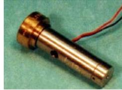
**Figure 2.** Single-jet device for micro-dispensing up to temperatures of 300°C.
