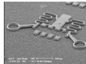
**Figure 24.** MEMS based metallic clampers for mechanical positioning and metal pads for electrical connections.
