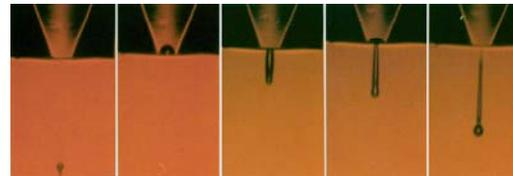
**Figure 1.** Sequence (left-to-right) of formation and ejection of a 50  $\mu$ m diameter droplet from a drop-on-demand inkjet device.
