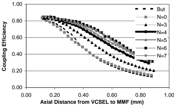
**Figure 18.** Coupling efficiency from VCSEL to MMF for different epoxy drop number N printed on pedestals.
