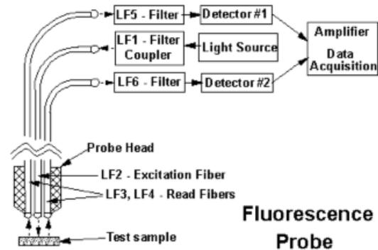
**Figure 26.** Schematics of a fluorescence probe and detection system.
