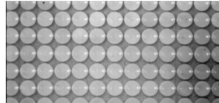
**Figure 6.** Printed array of 916 μm diameter microlenses on 1 mm centers with focal lengths of 1.10 ± 0.01 mm.
