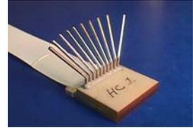
**Figure 3.** Array printing device, 1 inch wide, for micro-dispensing up to 10 different fluids.
