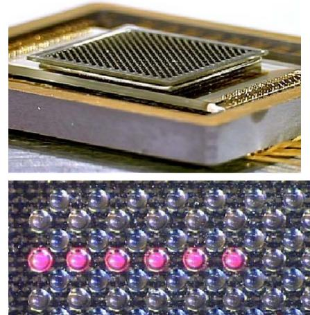
**Figure 14.** Smart pixel array module (top) and printed 250 μm diameter microlens array in module with VCSELs under 6 lenslets turned on (bottom). (Photo courtesy of Y. Liu & A. Cox of Honeywell)
