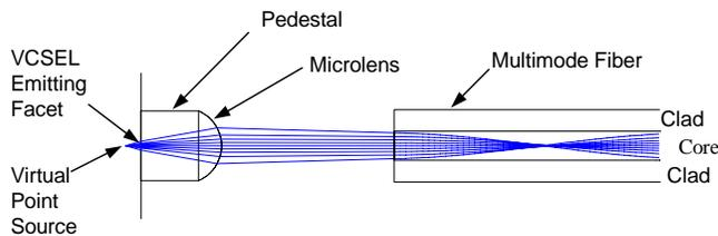
**Figure 15.** Integration of pedestal and microlens with VCSEL for light coupling to multimode fiber.
