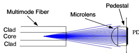
**Figure 16.** Integration of pedestal and microlens with PD for light coupling from multimode fiber to PD.
