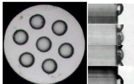
**Figure 13.** Array of 80  $\mu\text{m}$  diameter hemispherical indicator elements printed onto 480  $\mu\text{m}$  diameter fiber bundle, shown from above (left) and in profile (right). (Fiber bundle courtesy of B. Coleston and S. Brown of Lawrence Livermore National Laboratories.)
