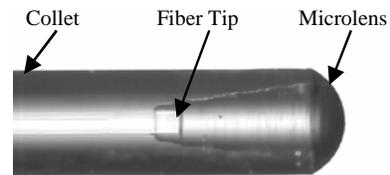
**Figure 10.** Fabricated lensed fiber.
