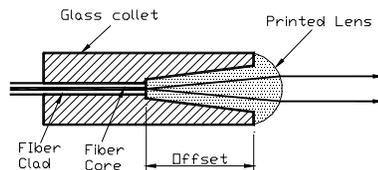
**Figure 9.** Concept of lensed fiber fabricated by inkjet printing.
