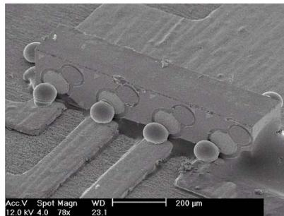
**Figure 21.** Direct PD die bonding using SolderJet®.
