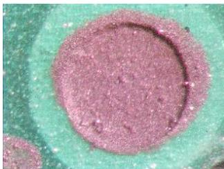
Chemo-resistive sensor, 350µm well.
