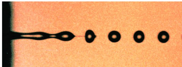
Figure 2: A 50: m jet of water breaking up due to Rayleigh instability into 100: m droplets at 20kHz.
