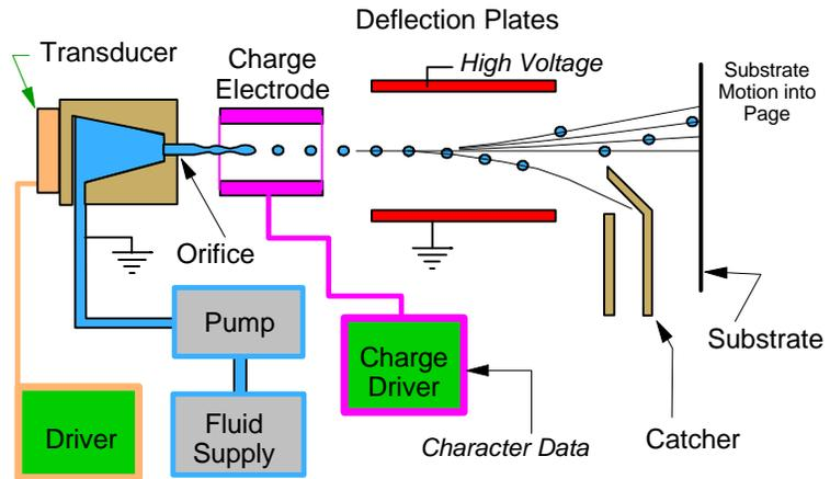
Figure 1: Schematic of a continuous type ink-jet printing system.
