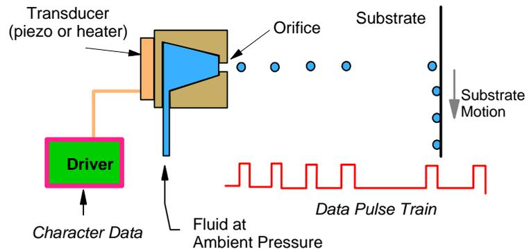
**Figure 3:** Schematic of a drop-on-demand ink-jet printing system
