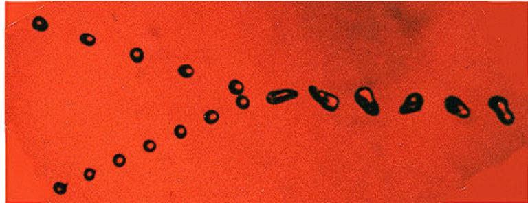
*Figure 5: Two streams of 120  $\mu$ m water droplets merging into a single droplet stream at 20kHz.*
