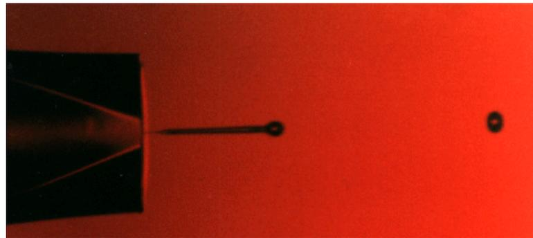
**Figure 4:** Drop-on-demand type ink-jet device generating 50 $\mu$ m diameter drops at 2kHz.
