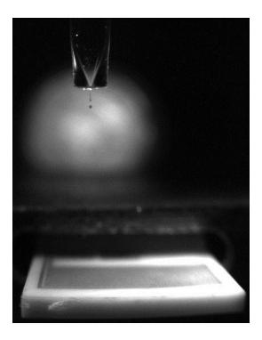
By dispensing small droplets of dilute solutions of explosive onto a heater, the materials vaporize rapidly and are carried away by a gas flow adjusted through a mass flow controller.
