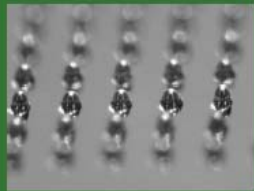
100 \mu m solder bumps printed onto pads at 400 bumps per second.
